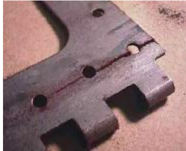
Indication of cracks running between attachment holes in a hinge
